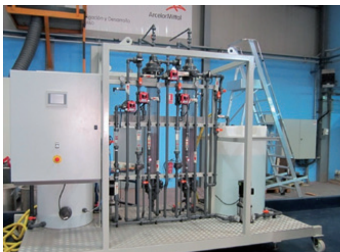
Pilot plant for different media filtration (Photo: AcelorMittal)
