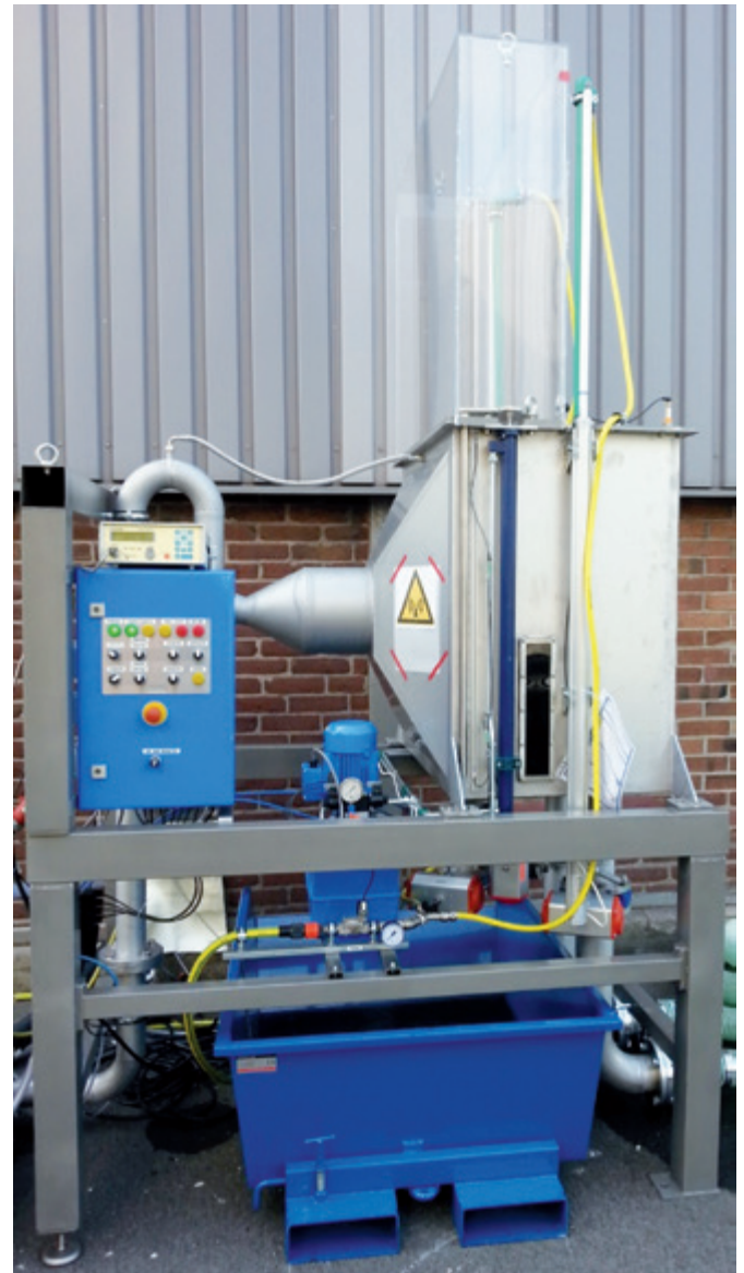
Strong field magnetic separator (Photo: BFI)
