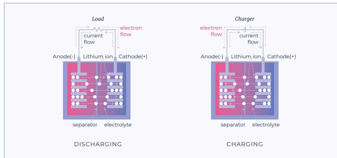
Figure 2. Charging and discharging of Li-ion cells
