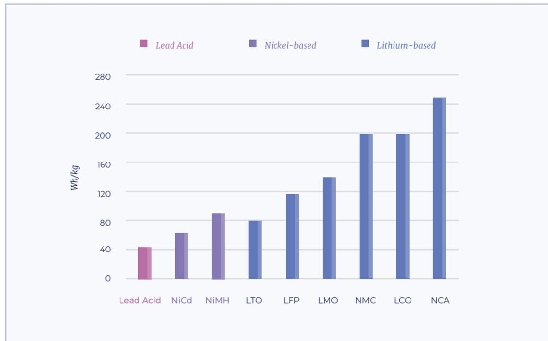
Figure 4. Specific energy for different batteries<sup>5</sup>
