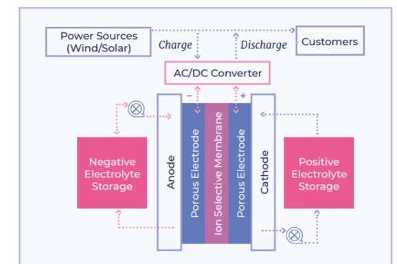
Figure 3. Generation of electricity in a flow battery
